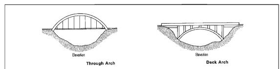
Arch bridges are comprised of convexly curved structural members that span openings and carry the roadway. Loads are transferred to piers or abutments at the end of the span through compression.
