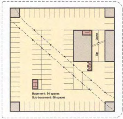
Basement & Sub-basement Plan
