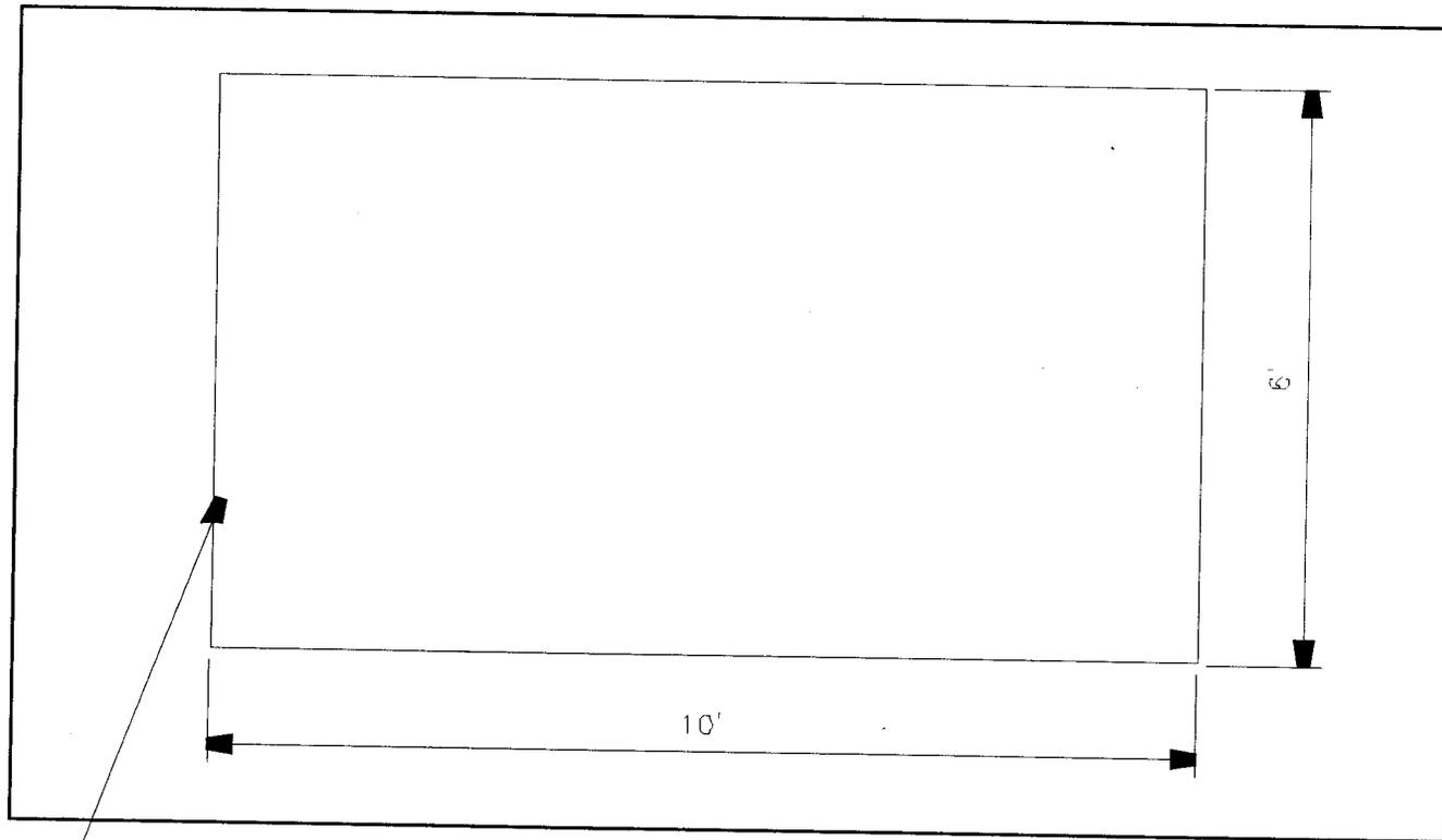
CONSTRUCT CONCRETE SHELTER PAD 5.5" MIN. THICKNESS, 3000 PSI PCC WITH 2" COMPACTED AGGREGATE BASE. SLOPE TO DRAIN TO CURB (NOT TO EXCEED 2%).
