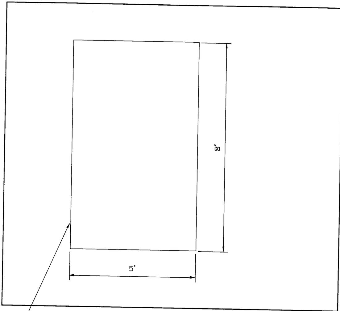
CONSTRUCT CONCRETE SHELTER PAD 4" MIN THICKNESS,
