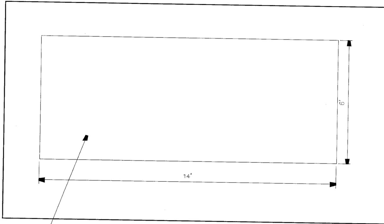
CONSTRUCT CONCRETE SHELTER PAD 8" MIN.
