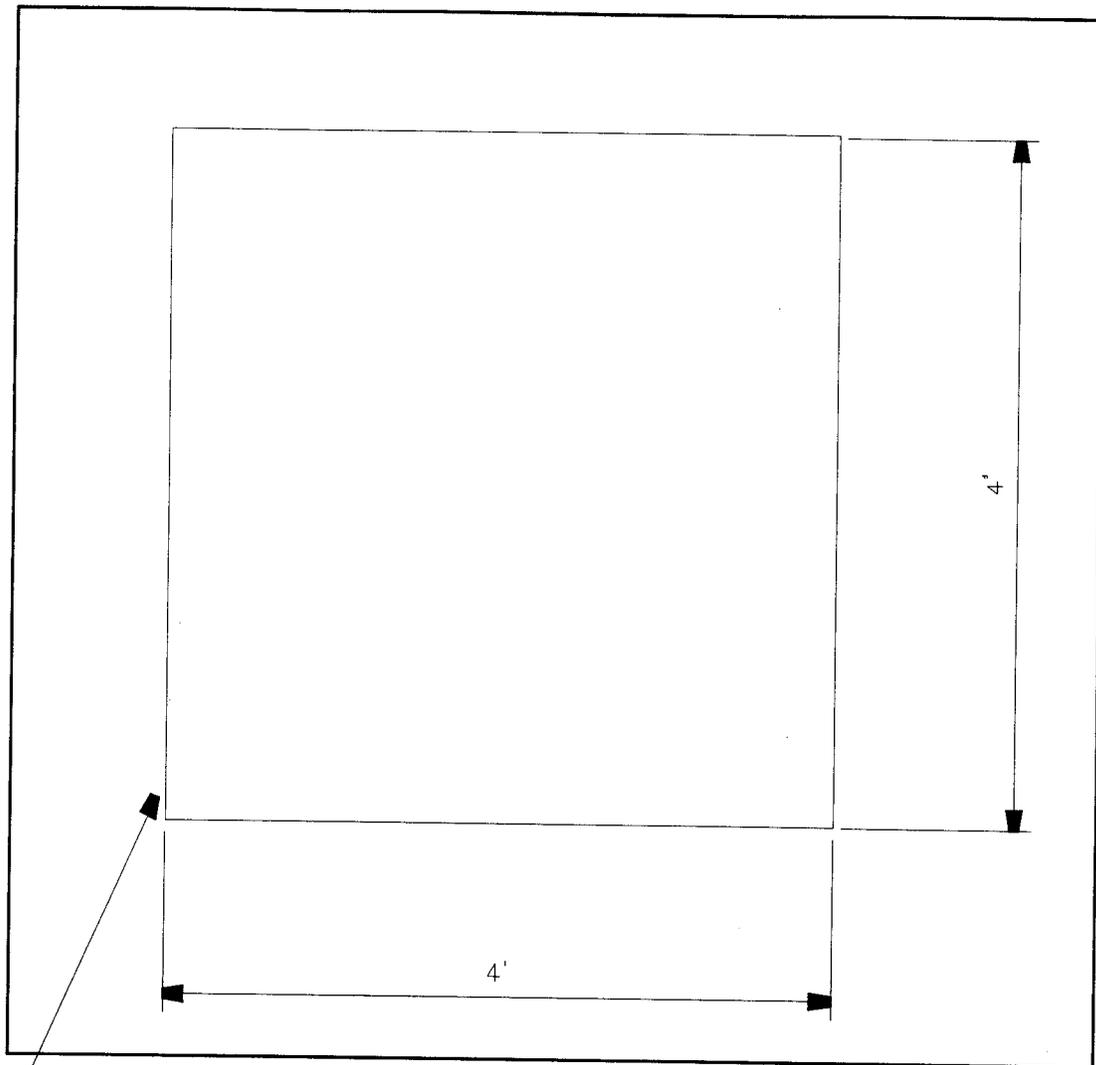
CONSTRUCT CONCRETE WASTE RECEPTACLE PAD 4" MIN. THICKNESS, 3000 PSI PCC WITH 2" COMPACTED AGGRERGATE BASE. SLOPE TO DRAIN TO CURB (NOT TO EXCEED 2%).
