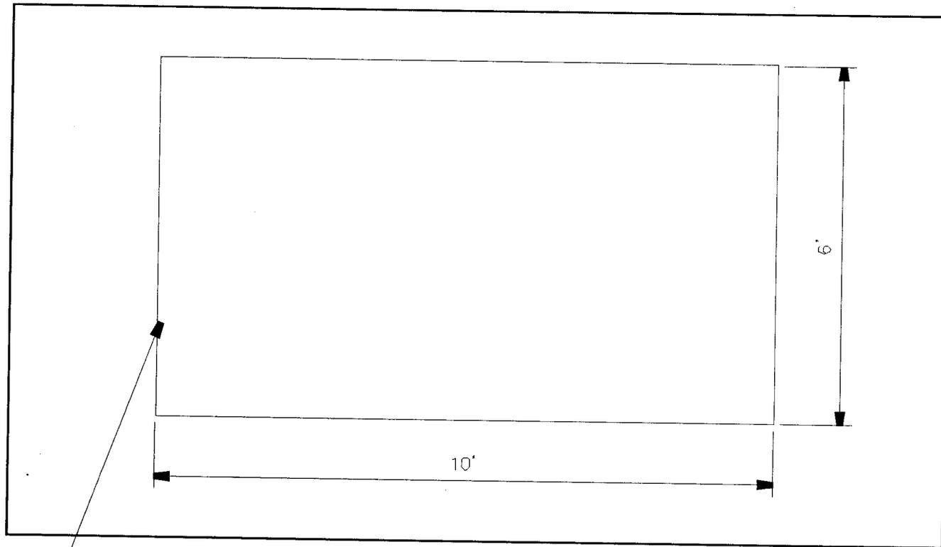
CONSTRUCT CONCRETE SHELTER PAD 5.5" MIN. THICKNESS, 3000 PSI PCC WITH 2" COMPACTED AGGRERGATE BASE. SLOPE TO DRAIN TO CURB (NOT TO EXCEED 2%).
