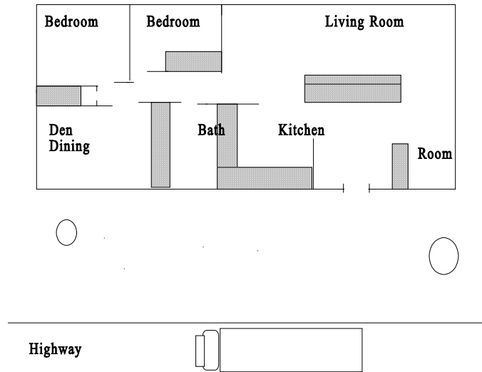
FIGURE 4.12 Use of Accoustical Architectural Design to Reduce Noise Impacts on More Noise Sensitive Living Spaces
