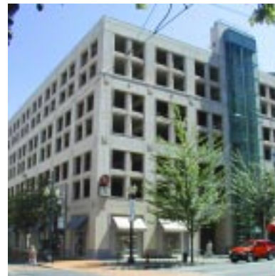
Recommended: Parking garage with ground-floor retail and window-scaled openings (SW Yamhill and 4th, Portland)
