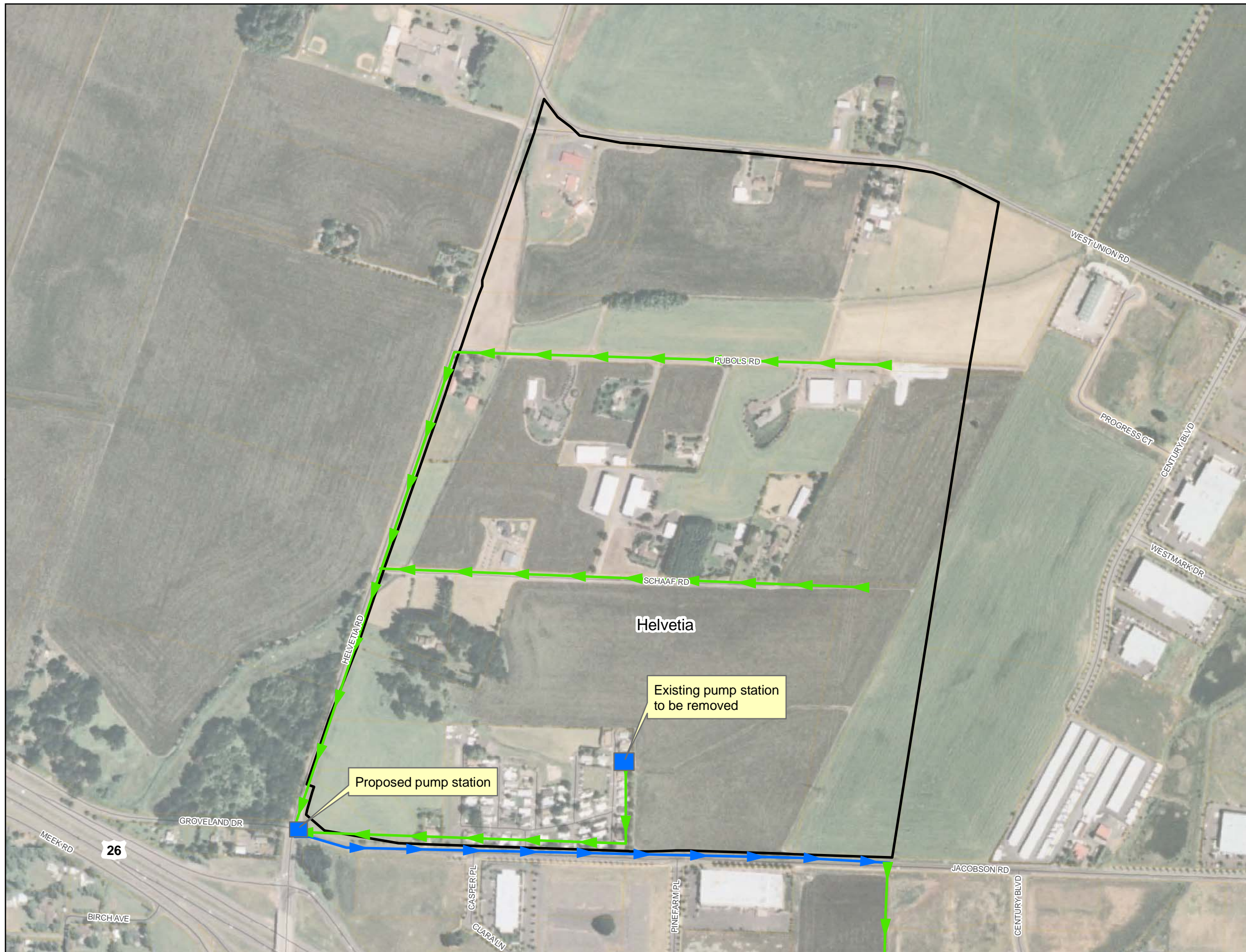
Figure 1 Helvetia Concept Planning Area Sanitary Sewer System Conceptual Alternative Evergreen/Helvetia UGB Concept Plans
