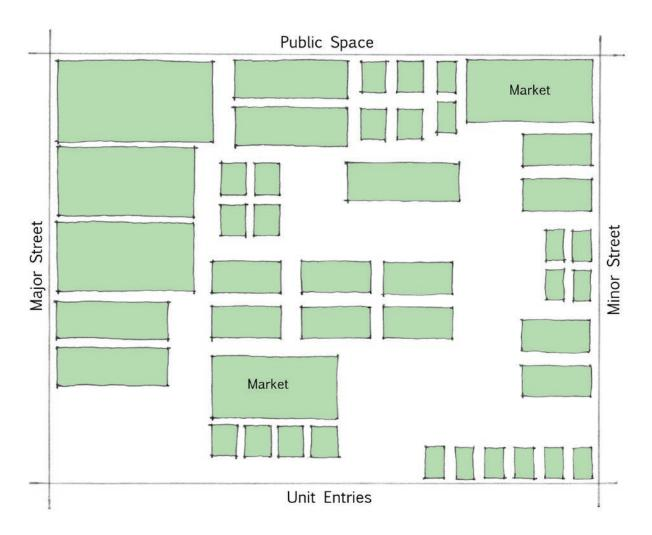
The markets present requirements different from the other commercial spaces; they are open air, but covered. It is likely that daytime cooling will be moderated by nighttime ventilation of mass; this is possible because the markets are on the ground floor, where the concrete structure will be exposed to provide the mass, and because the space will be completely open to breezes during the night. Other commercial spaces will need more active cooling methods.
