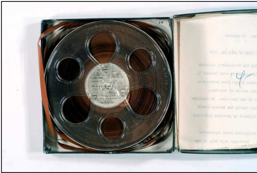
Photo 14 Reels with loose tape packs, damaged ends
