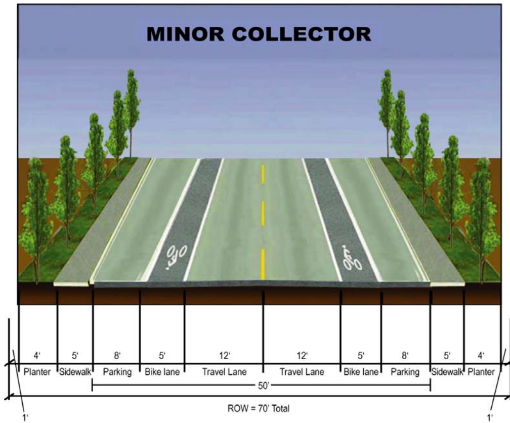
FIGURE 7-5 Typical Minor Collector Street Design Standard Criteria (Diagram shows 70' ROW, 2-lane configuration)
