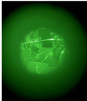
Figure 21: Photo of Infrared Light Leakage from Fiber
