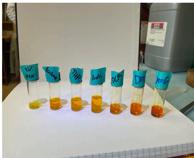
Figure 9: Optical properties of Compound 12 dissolved in different solvents.
