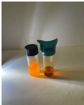
Figure 11: Aggregate induced emissions of Compound 12 in organic solvent (right) and inorganic solvent (left).
