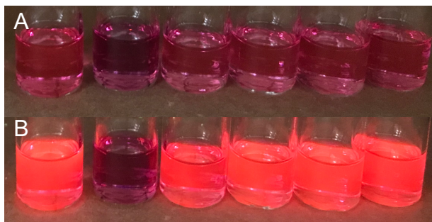
Figure 3.4. Screening of host-guest interactions of L_2 with aromatic small molecules. a – e are L_2 with 1,4-dimethoxybenzene, 1,3,5-trimethoxybenzene, xylenes, toluene, and benzene. (A) without UV radiation and (B) with UV radiation.
