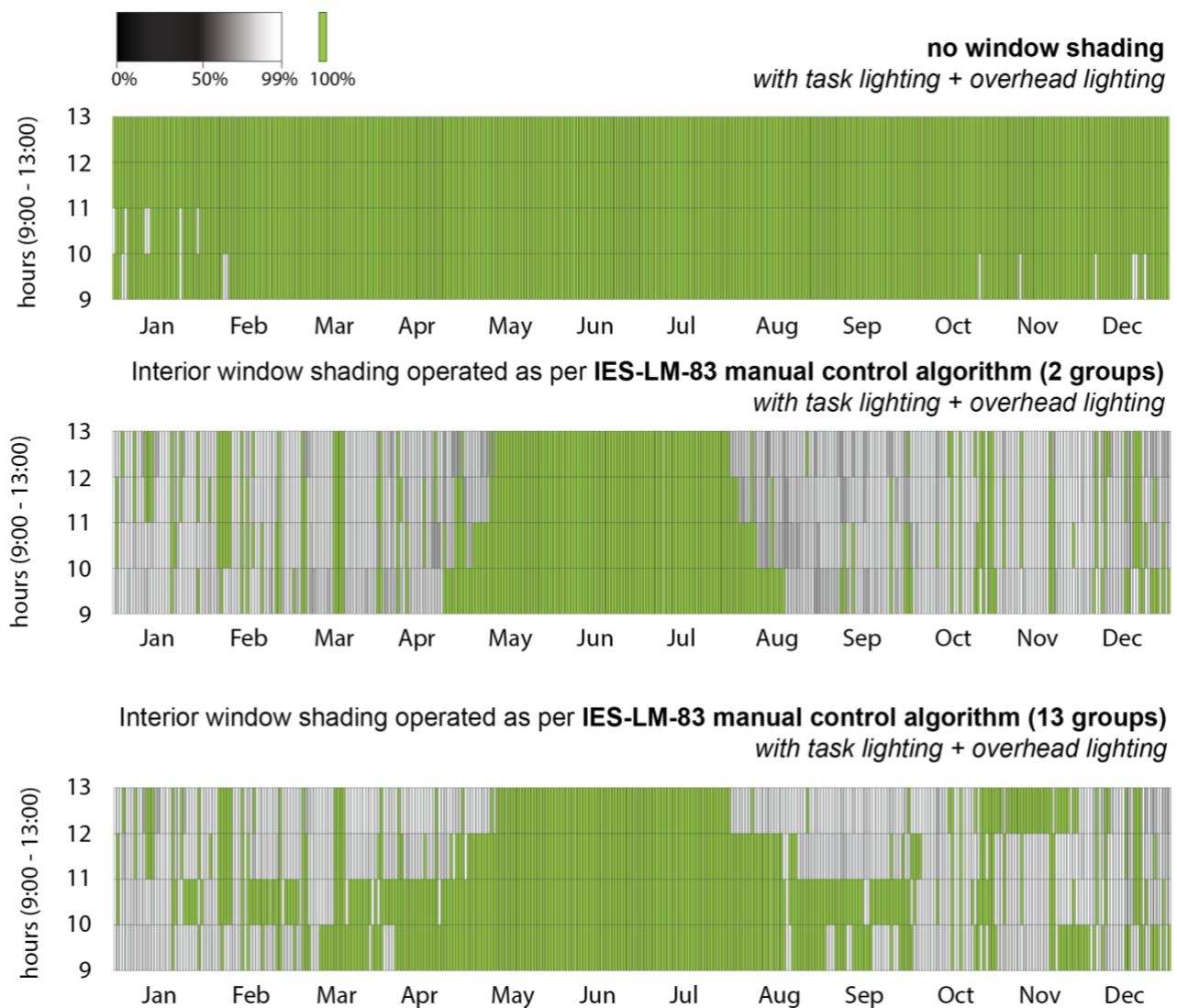
Figure 6: Percent of workstations that achieve WELL v2 (275 EML threshold) between 9am and 1pm between the three design scenarios (no window shading, IES-LM-83 2 window groups, and IES-LM-83 13 window groups)
