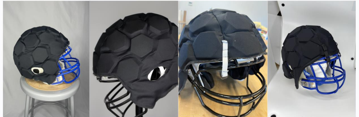
V.1 (Sewing) → V.2 (Hook & Loop Attachment) → V.3 (G-Hook Attachment) → V.4 (Bonding and Finished Edges)
