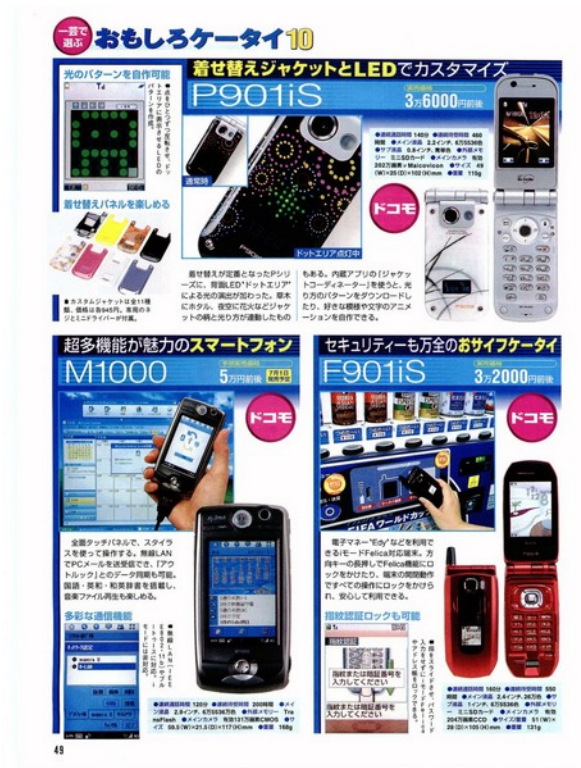
Figure 4.46: Unique keitai features such as customizable external LED display, “osaifu keitai,” and an early smartphone with touchscreen and WiFi. Shūkan ASCII , July 12, 2005, 49.
