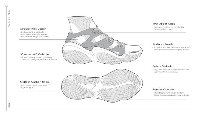
Fig. 52. Technical drawing of shoe with callouts
