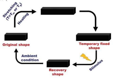
Fig. 32. Programming process of Shape-Memory Polymers
