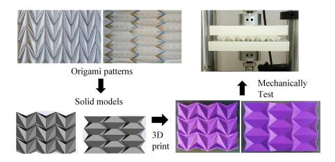
Fig. 34. Application of origami as a load-damping metamaterial
