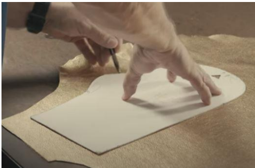
Figure 11. pattern and cut leather (1v1 Fight Gear, 2020)
