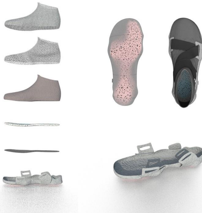
Figure 49. Exploded View and material breakdown for Training Footwear.
