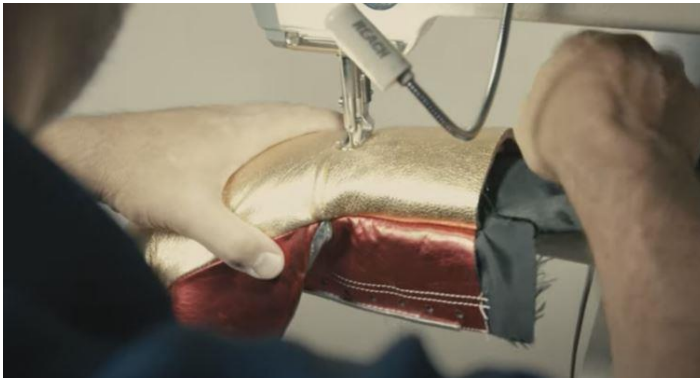
Figure 14. stitching palm onto lining (Iv1 Fight Gear, 2020)
