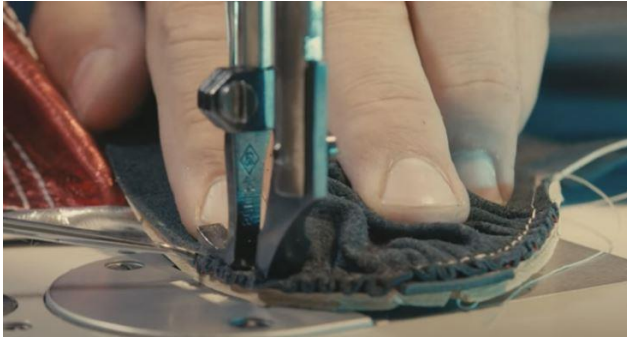
Figure 12. gathering and stitching knuckles and thumb (1v1 Fight Gear, 2020)
