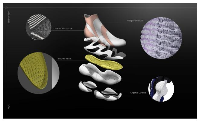
Fig. 51. Exploded view showing key elements of shoe design
