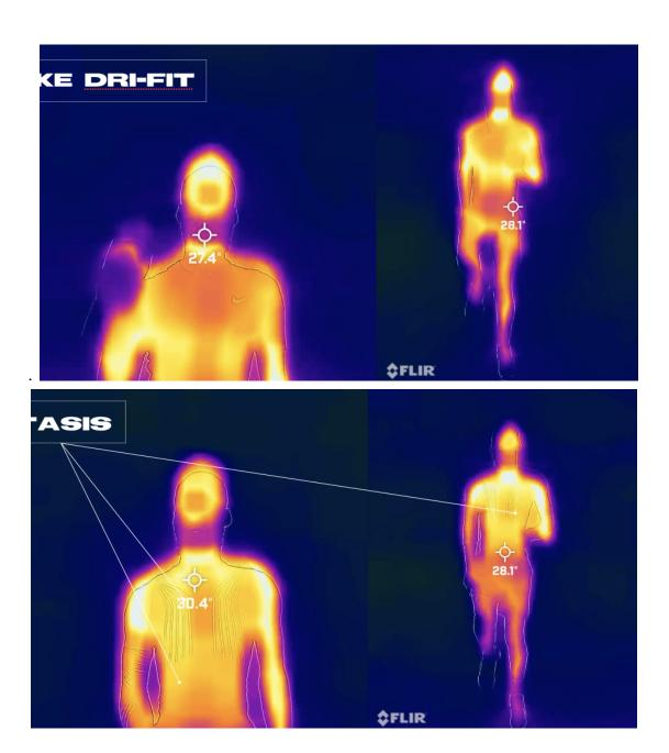
Figs. 70-71. Validation testing using FLIR thermal imaging
