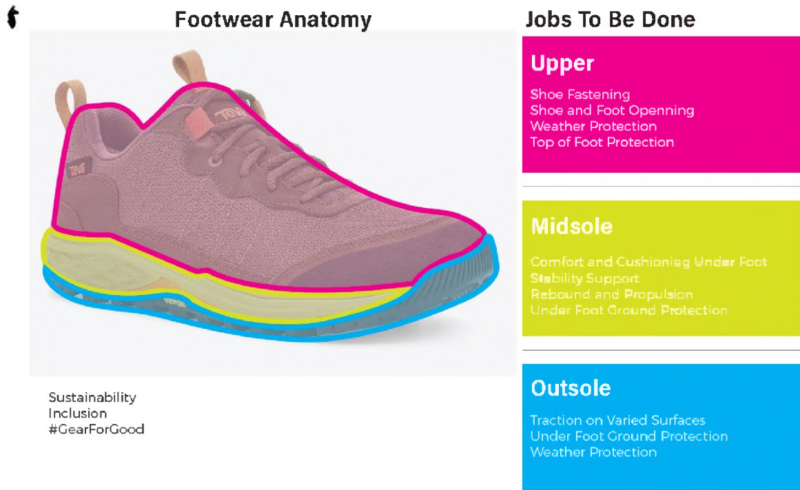
Figure 10. Display of exterior shoe anatomy (insole is inside shoe and not on display in this figure).
