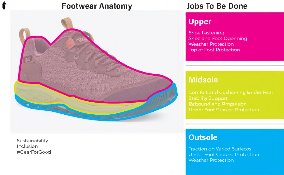
Figure 10. Display of exterior shoe anatomy (insole is inside shoe and not on display in this figure) (Hintze, 2021).
