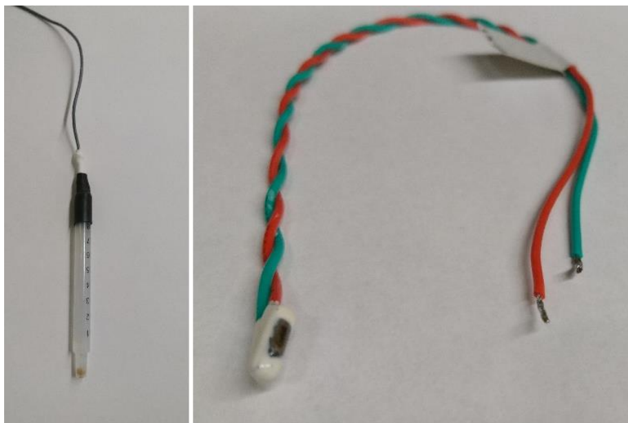
Figure B2. Reference electrode (left). Red and green colored wires connected to the functionalized ChemFET (right) indicate the source and drain connections, respectively.
