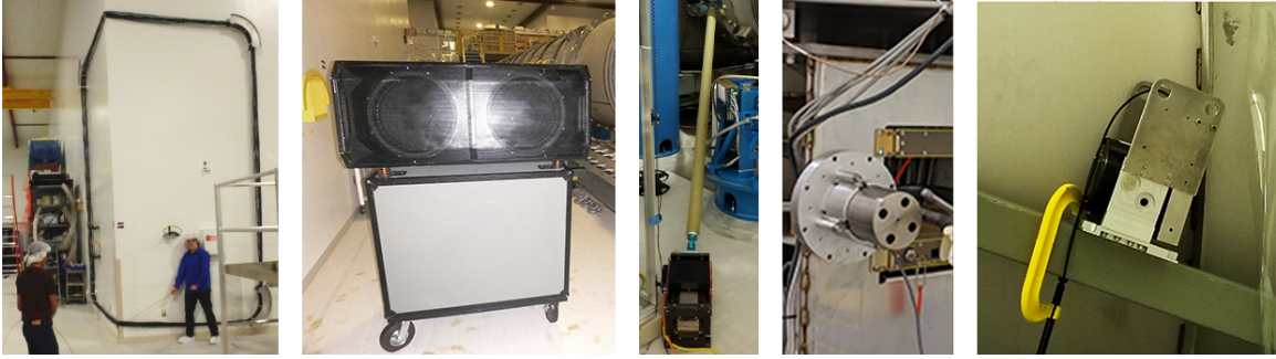
Figure 7. Injection equipment photos. From left to right: wall-mounted magnetic field injection coil; 14-in. speakers; APS 113 shaker connected to the door of a vacuum chamber by a rigid fiberglass rod; modified Piezosystem shaker clamped to an electronics rack; modified B&K shaker clamped to a beam tube support.
