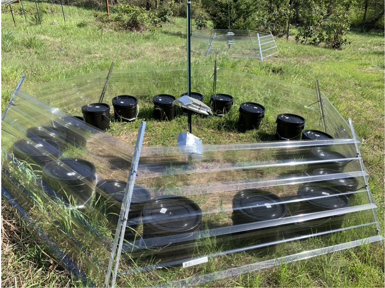
Figure S4.2. Modified passive warming chambers used to heat macroplots in this study. Design and dimensions based on (Godfree 2011). Chambers were constructed using PALRAM® polycarbonate panels, angle aluminum and zipties. We modified the original design using eighteen 3.5 gallons (63 gallons of water per chamber) buckets as thermal mass immediately inside the perimeter of each chamber.
