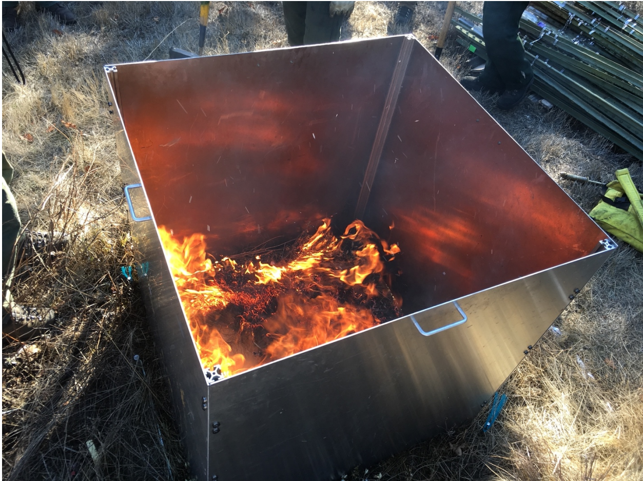
Figure S3.1. Burn boxes are an alternative to full-pasture prescribed fire that have been successfully used across western grasslands to reproduce typical prescribed fire effects at a small scale (Sharrow & Wright 2018; White & Currie 1983). Our burn box was constructed of four 1 m by 1 m aluminum panels that bolt together using rails as seen above. The box can be disassembled for transport and has a handle on each panel.
