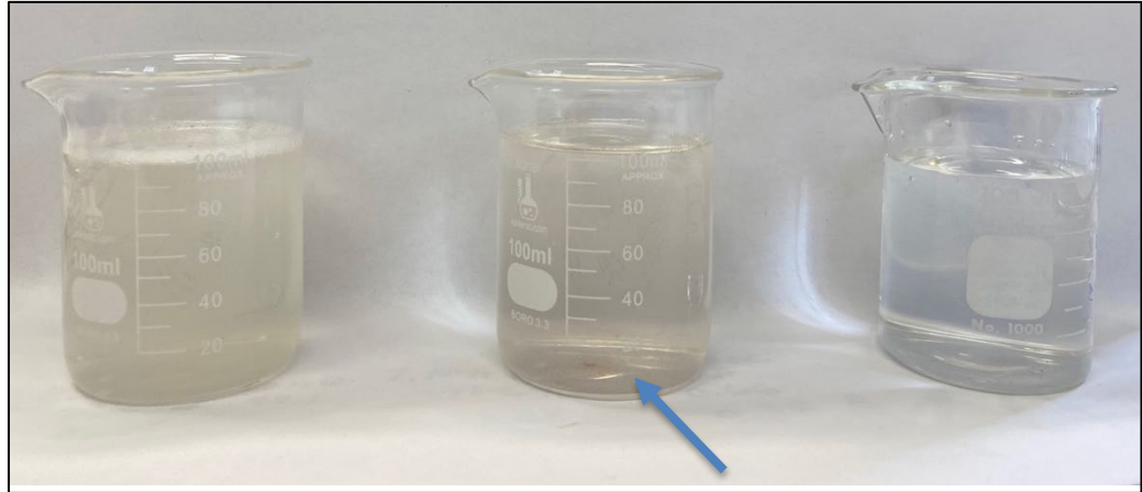
Figure 34: Three 100 mL beakers containing (left to right) control graywater, graywater after 7 days in Sco 16-32 mm samples, and tap water.
