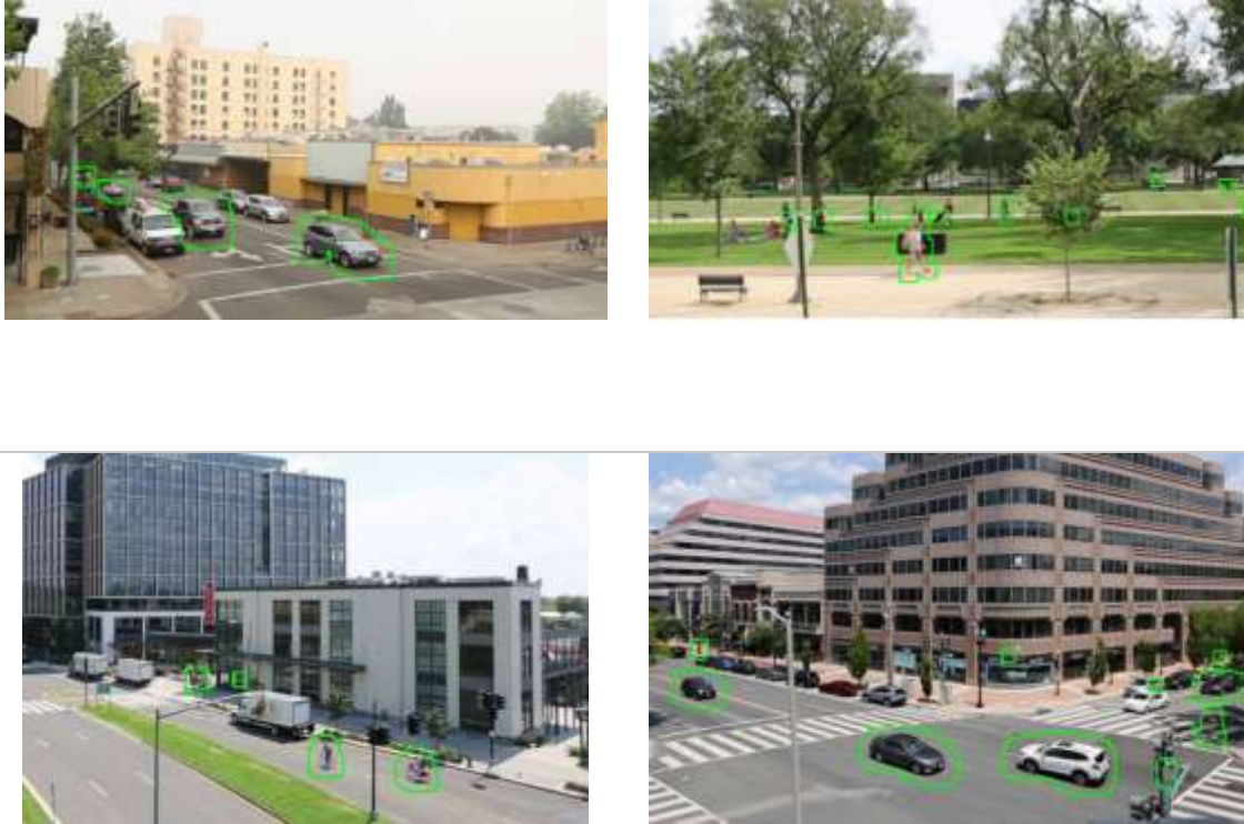
Figure 2. Examples of 4 views when the code was applied to videos. The green boundary line around the objects show the dynamic object which can be either cars, people or natural elements.
