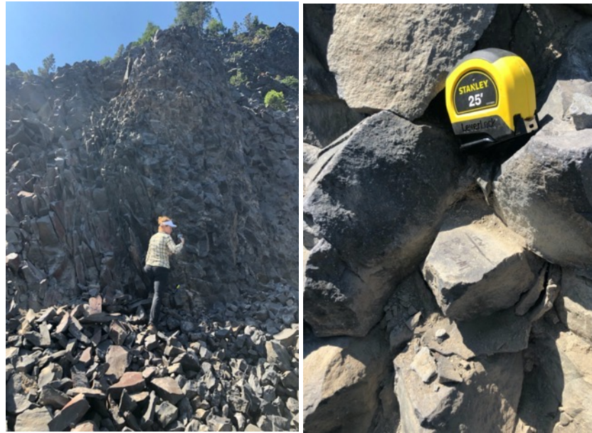
Figure 12: Cube joints at Hogg Rock, at outcrop scale (left) and at joint scale (right)
