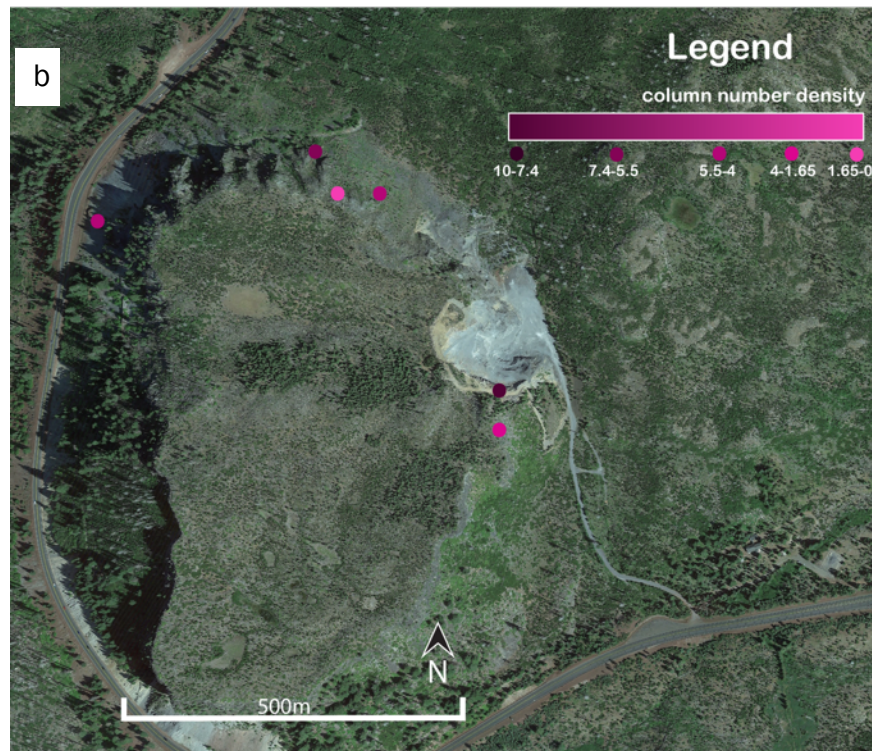
Figure 22: Lateral distribution of number density of pseudo columns across Hogg Rock. A) Histogram showing the distribution of number densities, with x-axis representing the joint density (1/m), and y axis representing number of outcrops in a given bin. The bins edges are at 0 m -1 , 1.65 m -1 , 3.9 m -1 , 5.5 m -1 , 7.4 m -1 , and 10 m -1 . B) Aerial image of Hogg Rock, with dots on areas where the joint density of pseudo columns was measured. The colors of the dots correspond to the bins in the histogram. The lightest pink represents the lower number density measurements, and dark pink represent highest number densities.
