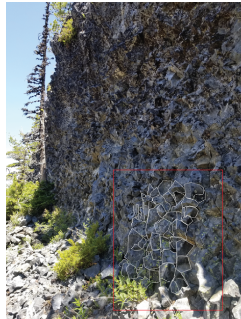
Figure 13: Schematic of how we measured joint density. For a given area (red box) we counted the blocks (cubes) present (white outlines)
