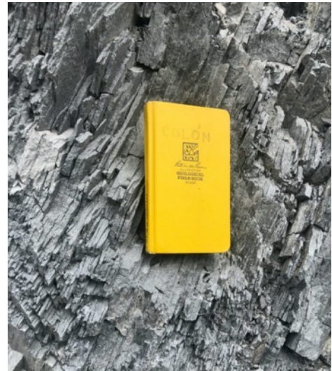
Figure 16: Smaller scale platey fractures at Hogg Rock. Note that these sets also have a preferred orientation, but they occur between sets of other fractures.
