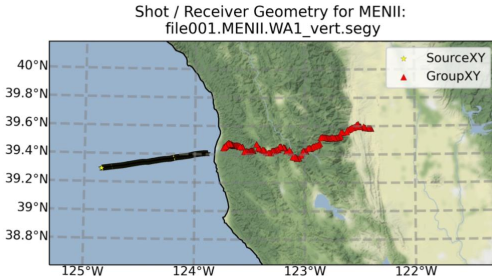
Figure A-2: Example of the extraction and plotting of shot / receiver geometry on a file-by-file basis
