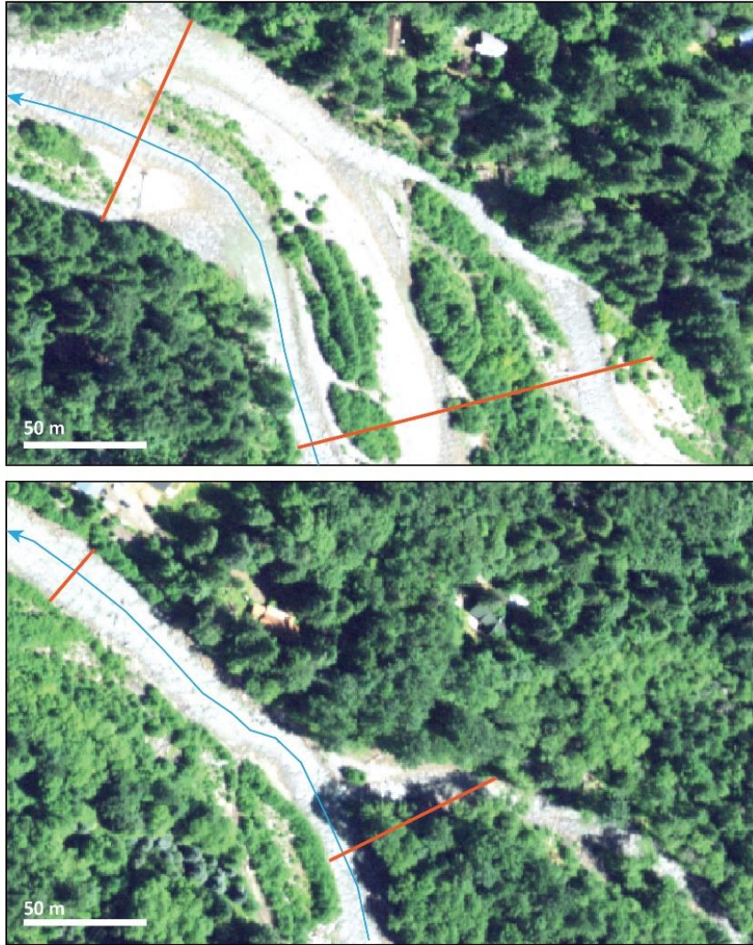
Figure 13: Examples of centerline (blue) and transects (orange) measuring the active channel width in multi-threaded reaches.
