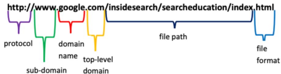
Figure 5.1. Basic anatomy of a URL ( Technology for Librarians 101: Anatomy of a Web Address , 2014).
