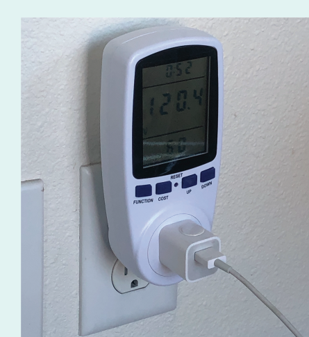
Digital Power Monitor Meter Usage Energy Watt Amp Volt kWh Electricity, manufactured by Zhengzhou Paiji Technology
