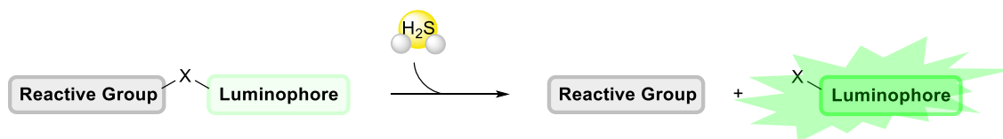
Figure 6.1 General principle for turn-on reaction based H 2 S probe design: a luminophore is quenched, and upon selective reaction with H 2 S or HS - , the luminophore is released and an optical response is observed.
