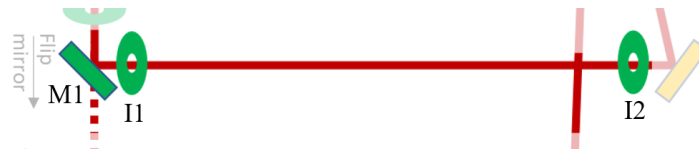
Fig. A.20. Alignment down table. M1 aligns beam through I1 and I2.
