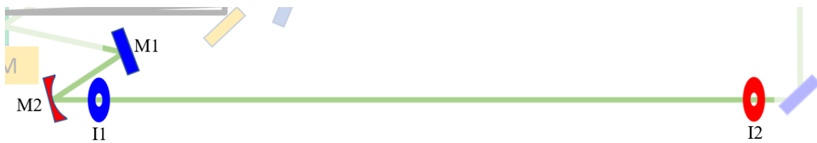
Fig. A.34. Alignment down table after SLM. M1 and M2 align the beam through I1 and I2, respectively.
