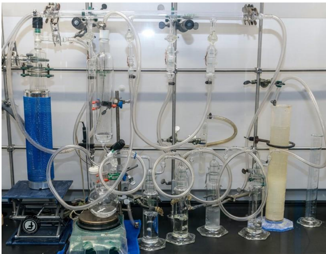
Figure G.1 Assembled glassware for synthesis and purification of COS
