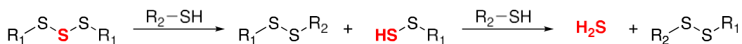
Scheme A.17 Mechanism of H 2 S release from organic polysulfides including DATS in the presence of thiols. We note the presence of a pendant allyl group likely complicates the mechanism of H 2 S release from DATS .
