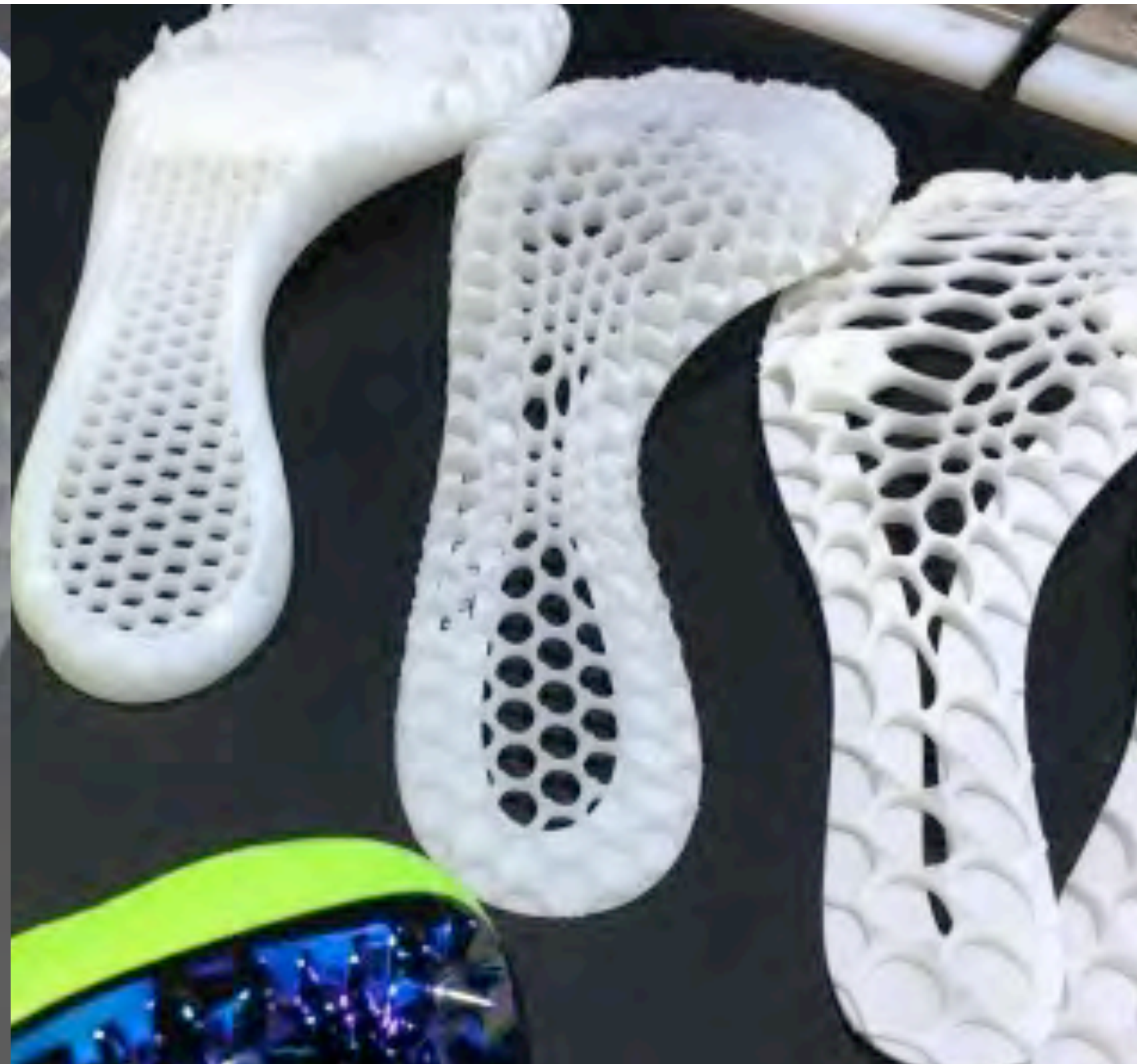
Laser cut upper, heat press TPU Injection molding for midsole 3D printed spike plate
