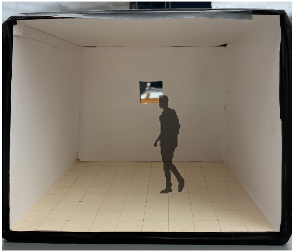
Figure 5: Canson paper clad interior + daylight factor grid on ground plane. Light meter hole.
