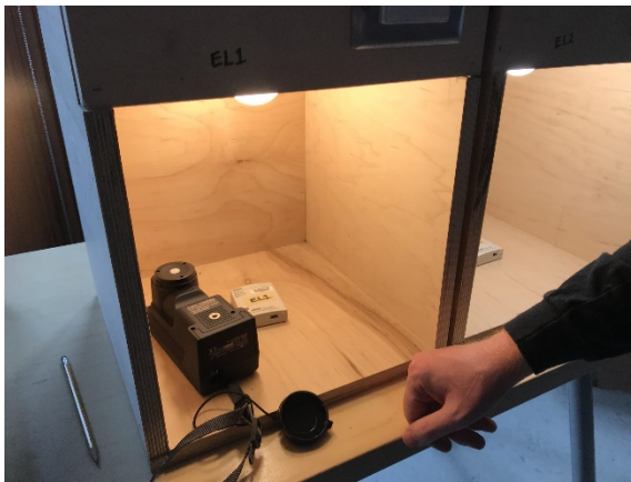
Figure 9: Measuring the spectral light intensity in each light box.
