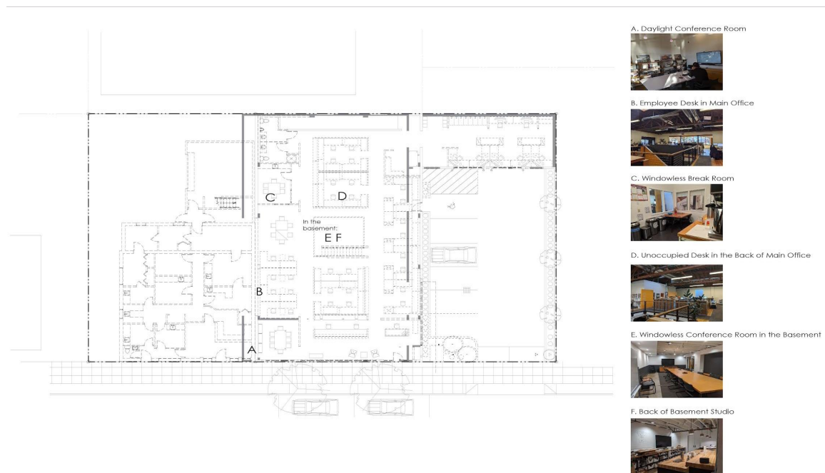
Figure 1: Existing building floor plan of Scott Edwards Architecture with bacteria locations marked.
