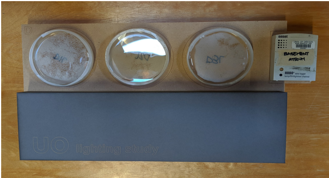
Figure 6: Tray at each location with three trial petri dishes, 3 control petri dishes covered by a black box, and a hobo data logger.
