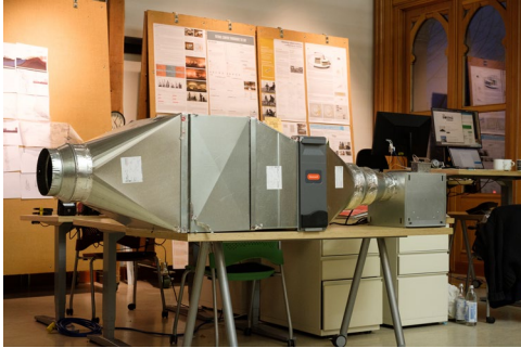
Figure 18: Ductwork serving as the chamber for the control experiment. Source: (Marsie Surguine 2019)
