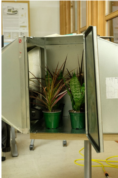
Figure 21: Controlled chamber testing with multiple Sanseveria Robustas (left) and a combination of Sanseveria Robustas and Dracaena Marginata Coloramas (right) Source: (Marsie Surguine 2019)
