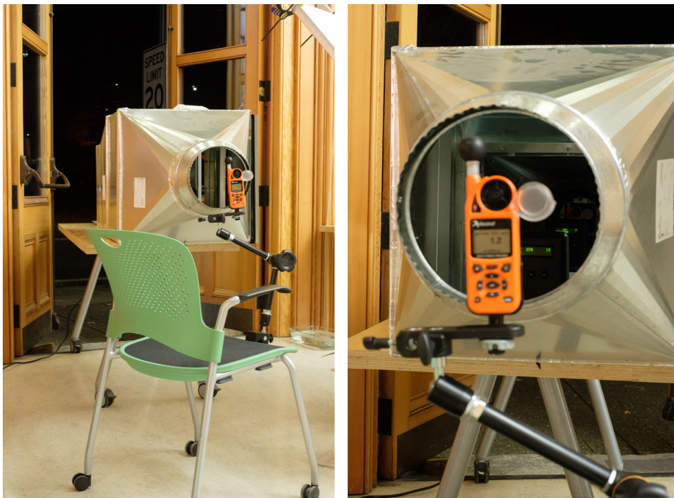
Figure 19: Controlled chamber testing set-up. Source: (Marsie Surguine 2019)
