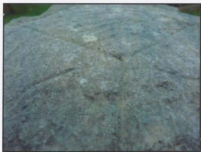
Detail of loose calcite granules on top of monument post-treatment
