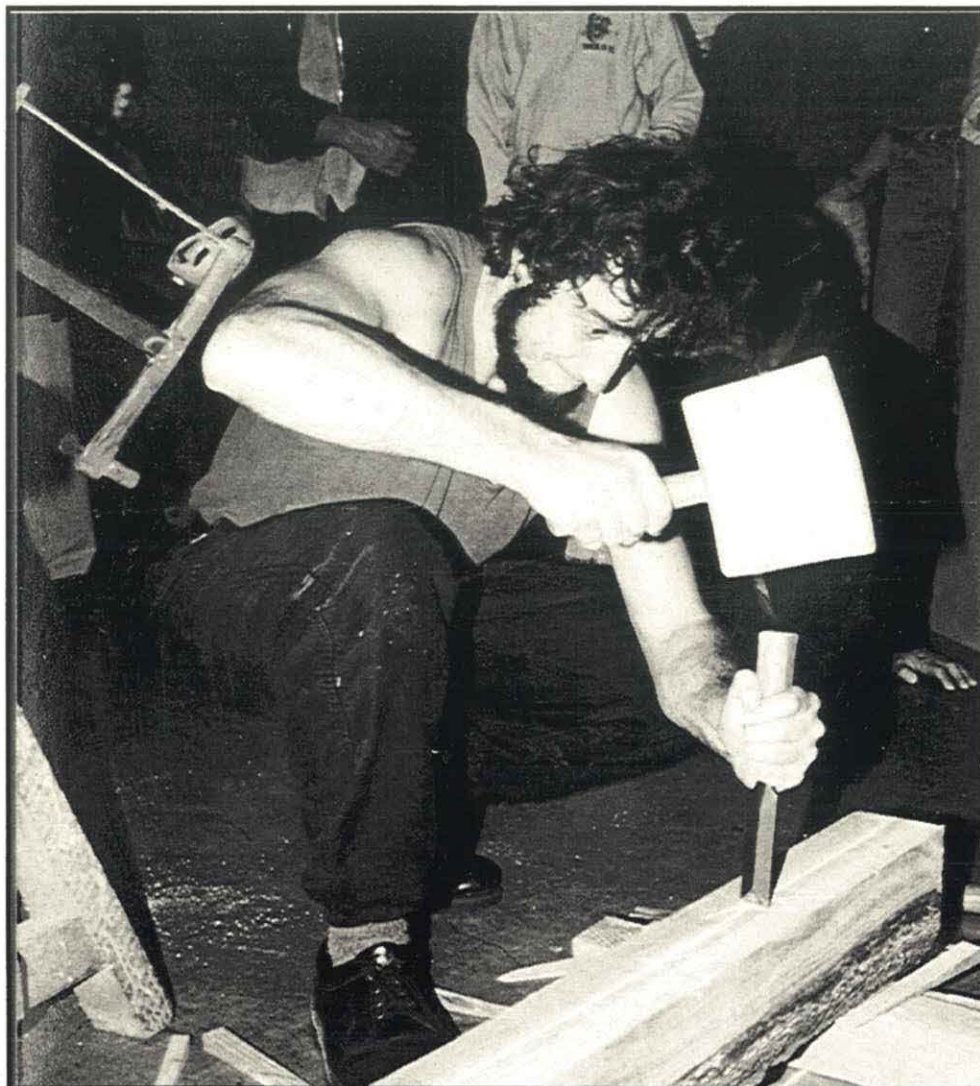
Frederic Brillant cutting a mortise during the demonstration at the U of O, which can be seen next page.
