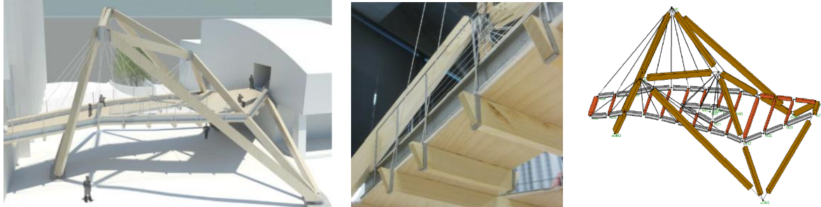
Figure 3. Space Truss Bridge (1 st Place), Architecture students: Nathan Houck, Greg Sagherian, Robert Yamnitz, Elane Yiu, Engineering students: Bethany Lopez, Daniel Mourad, Ryan Turner, Samson Wong. Physical models at 1/4" and 1"=1'-0", left; digital structural model in RISA 3D, right.
