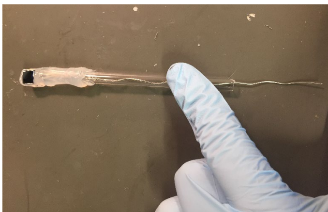
Figure 7. Electrode preparation a) Silicon wafers before cleaning. b) Back contact on wafer formed using Ga-In eutectic and a Cu-Sn wire. c) Fully made electrode.
