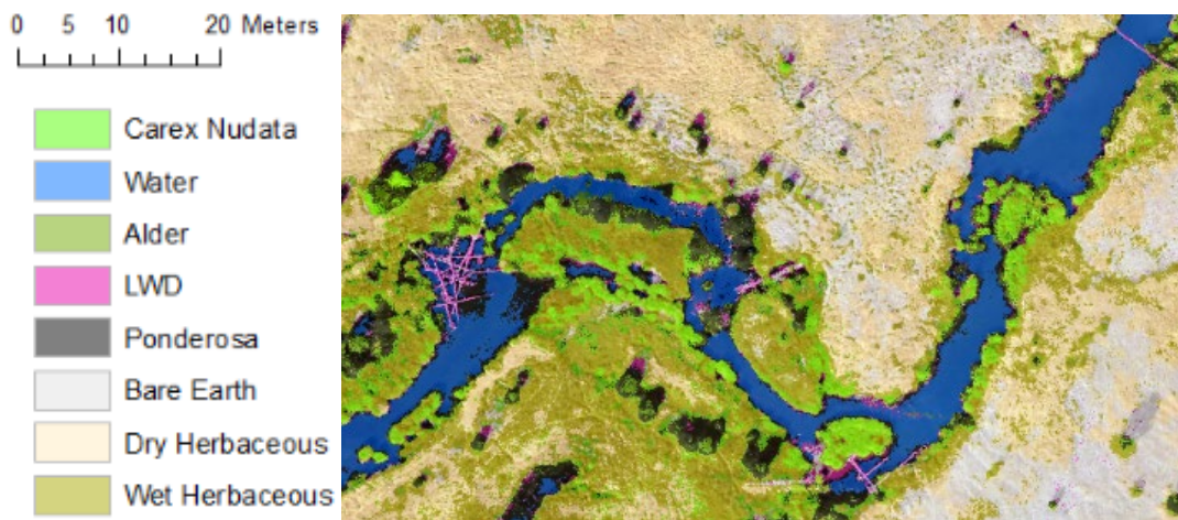
Figure 13: Example of classified imagery in Oxbow Conservation Area. The classification performs best for differentiating dry and wet herbaceous material, water, and large woody debris.
