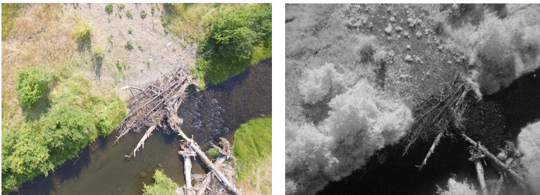
Figure 5: Example of unprocessed JPEG images taken with the Phantom III Pro FC300X camera (left) and modified Canon A480 (right). The RGB image at the left can be subsequently broken down into its 3 constituent bands of visible light and merged with the NIR image to produce a 4-band raster stack.
