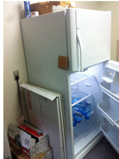
FIGURE 3.7. Left: Magnetometer plot at EY during O1 showing periodic glitches followed by temporarily elevated fields. Right: The culprit.
