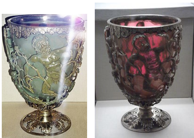
FIGURE 1.2. Dichroic phenomena due to nanoparticles in the Lycurgus Cup. The cup, made entirely from glass (including the cameo) appears green when light is reflected from its surface (left) but red when light transmits through it (right). Images by user Johnbod on Wikimedia Commons, copyright CC-BY-SA 3.0.
