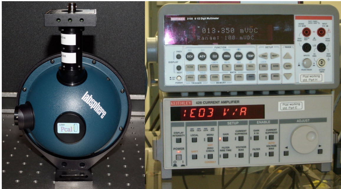
FIGURE 3.16. Gold Standard setup showing the power sensor mounted on an integrating sphere with Keithley Model 428 programmable current amplifier and Keithley Model 2100 digital multimeter.
