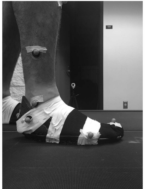
● MOTION CAPTURE WITH 3D PRINTED COMPONENTS THE BOWERMAN SPORTS SCIENCE CLINIC RAN WITH MOTION SENSORS BAREFOOT/ WITH NIKE METCONS/ THEN WITH 3 DIFFERENT 3D PRINTED FOOTWEAR VARIATIONS TO VALIDATE DESIGN DIRECTION
