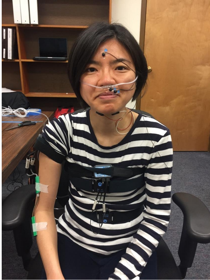
Figure 3. Respiratory belt transducer and nasal cannula arrangement.
