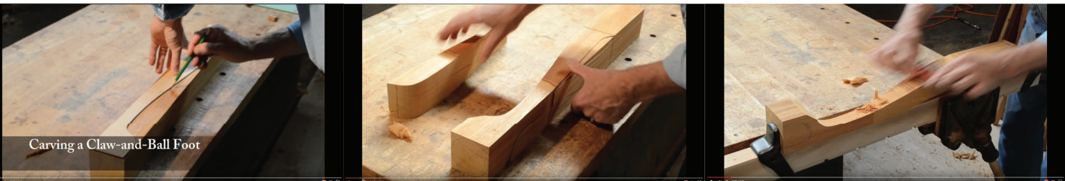
FIGURE 4.21 Stills from carving a claw and ball foot. https://www.youtube.com/watch?v=VcRgZF2trE
