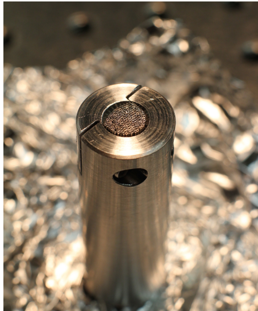
FIGURE 5.3. Strontium oven collimation nozzle
