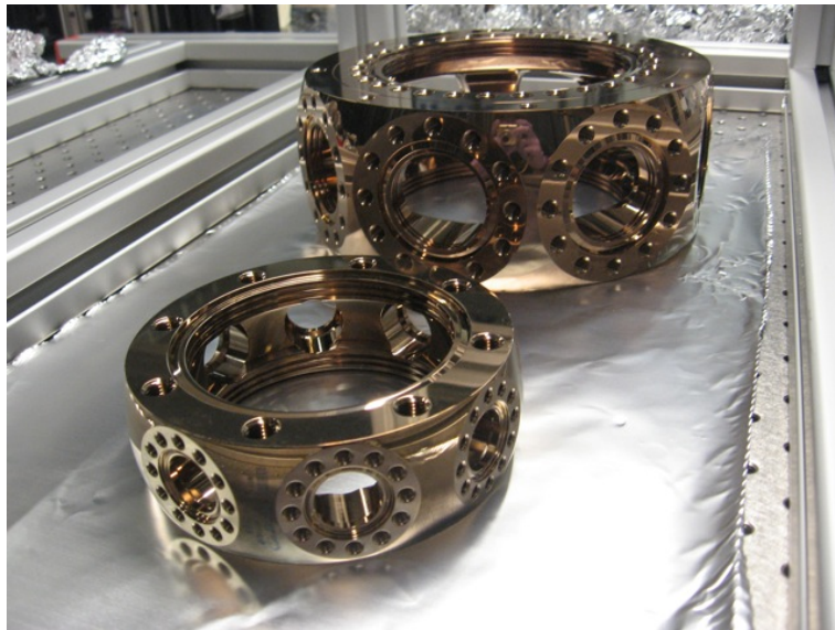
FIGURE 5.11. Vacuum chamber 4.5" and 6" spherical octagons, after air pre-bake
