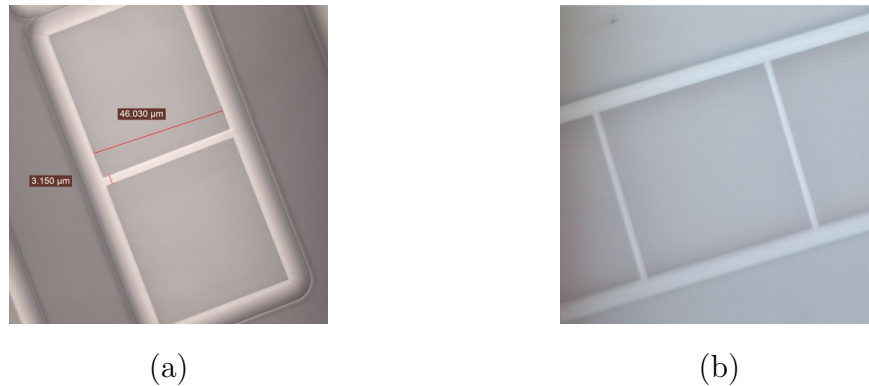
FIGURE 5.5. Optical images of (a) a ( 45\mu\text{m} \times 3\mu\text{m} \times 100\text{nm} ) silicon nitride beam and (b) arrays of beams fabricated by using the process shown in Fig. 5.4.
