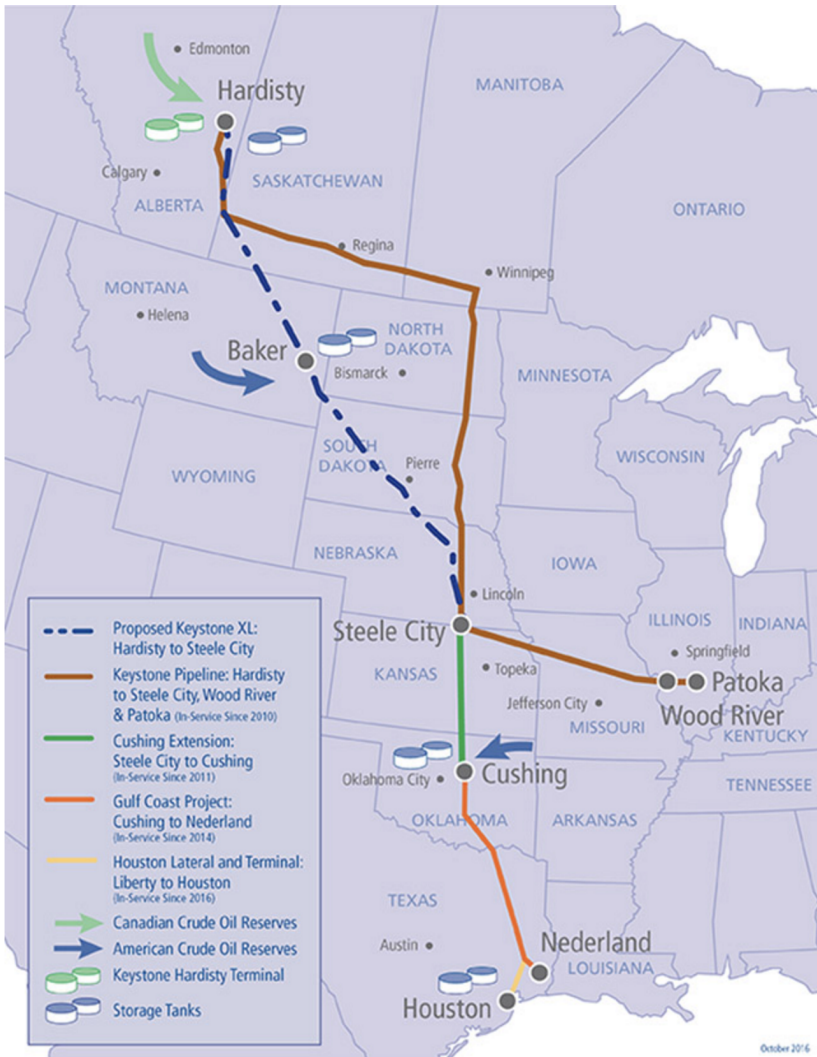
Figure 1: TransCanada’s map showing Keystone XL’s proposed routing as a broken line between Hardisty, Alberta and Steele City, Nebraska. The proposed pipeline travels through Alberta and Saskatchewan before going to Montana, South Dakota, and Nebraska. The other lines on the map depict already-completed pipelines in TransCanada’s network.
